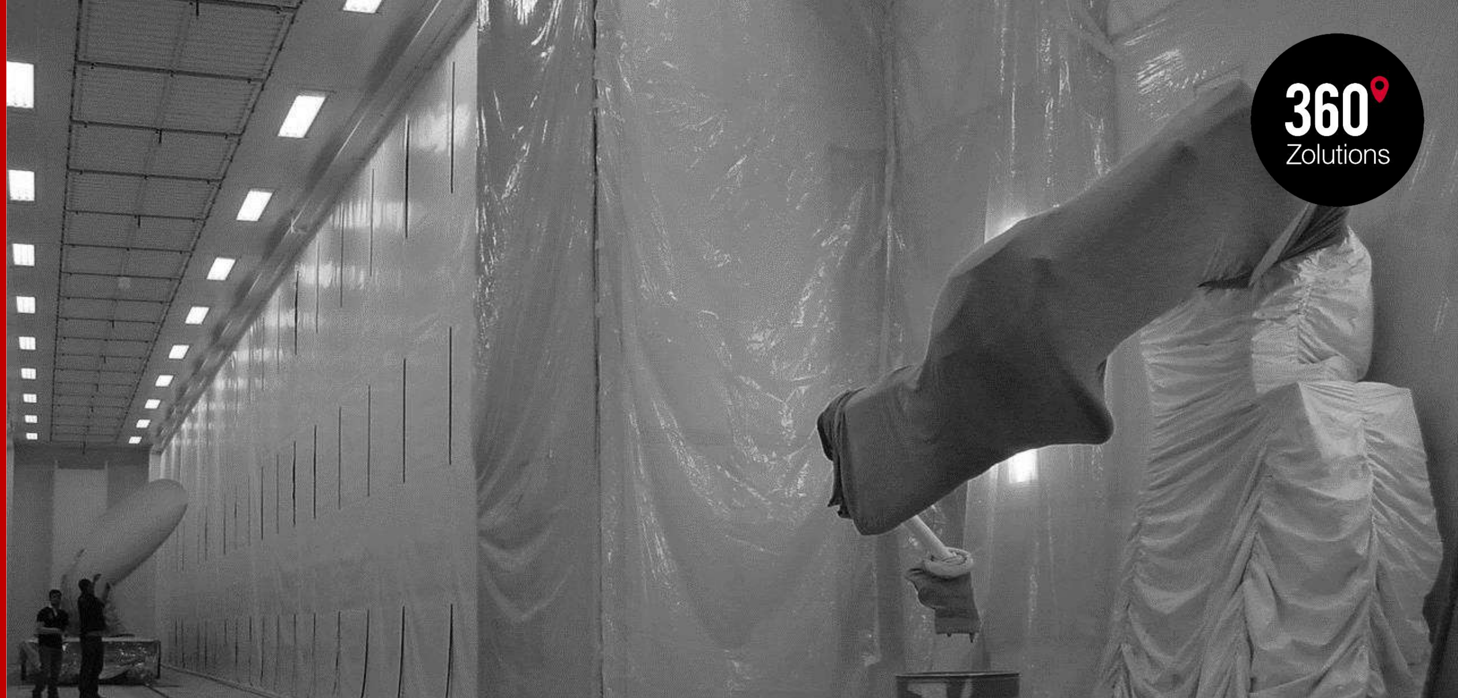
Painting cobots to reduce application time and overspray
